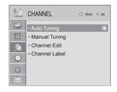
Use Channel Menu options to run Auto Tuning and edit the channel lineup, as necessary.
